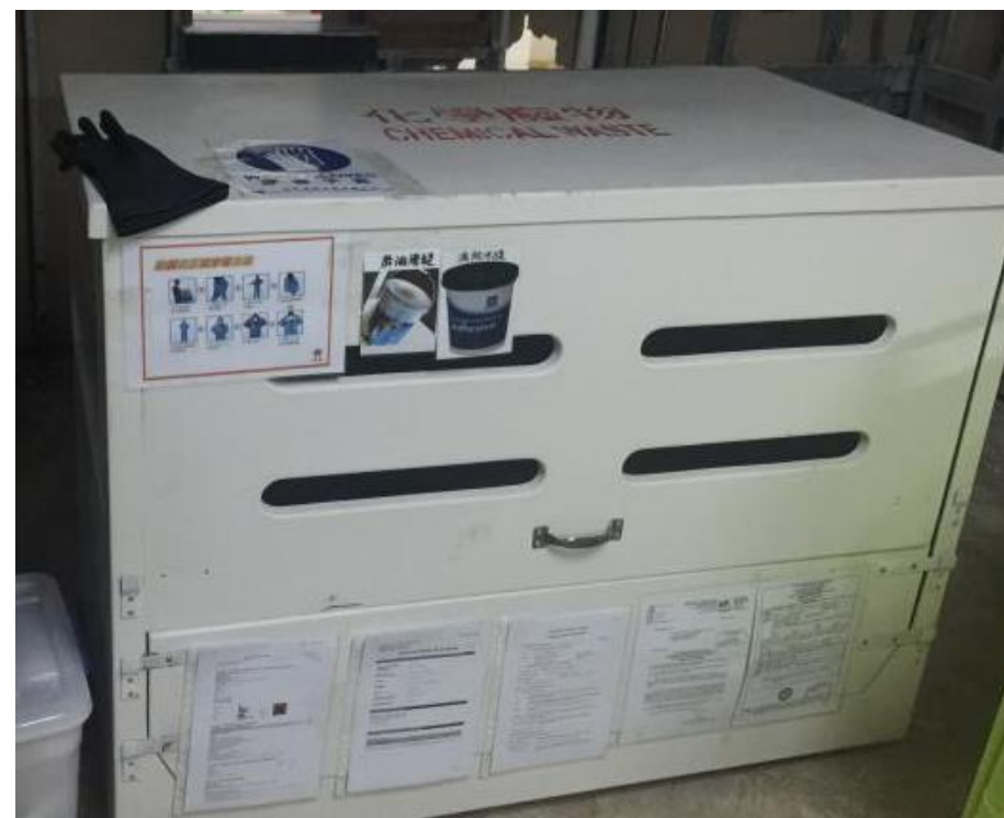
Chemical storage with chemical waste disposal license and MSDS displayed
